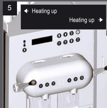
Machine heats up. All buttons flash in white.
